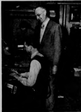
Every weekday morning copy is sent to the printers, the Leeland Type Setters, Mr. Howard Leeland, proprietor. Seated at the linotype machine is Earle Martin, setting some "Albrightian" copy, supervised by Mr. Leeland. In the rear is Bill Lochman making up some page forms.
