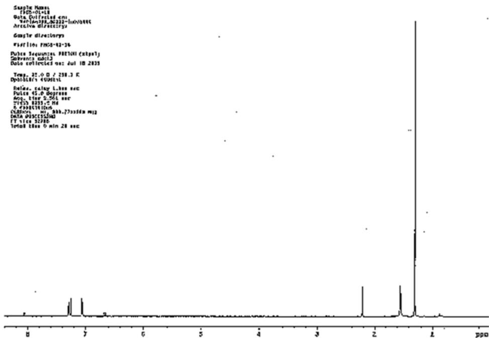
Figure 1.  $^1\text{H}$  NMR spectrum of *N,N*-di-(4-*tert*-butylphenyl)-*N*-(2-pyridyl)amine.
