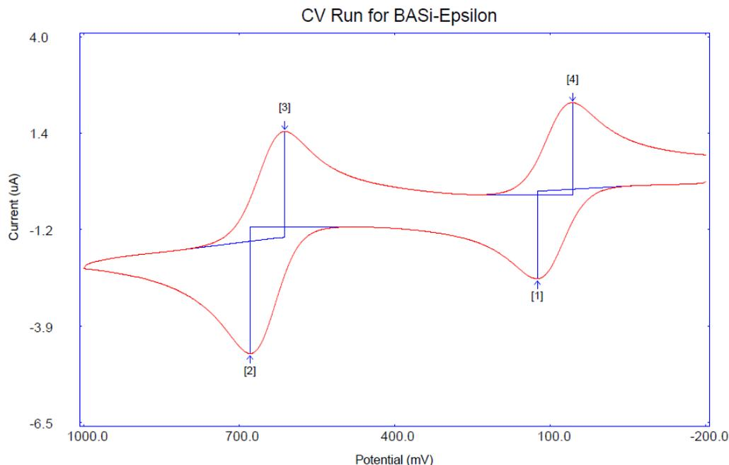
**Figure 3. Cyclic voltammogram for *N,N*-di-(4-*tert*-butylphenyl)-*N*-(2-pyridyl)amine with ferrocene internal standard.**
