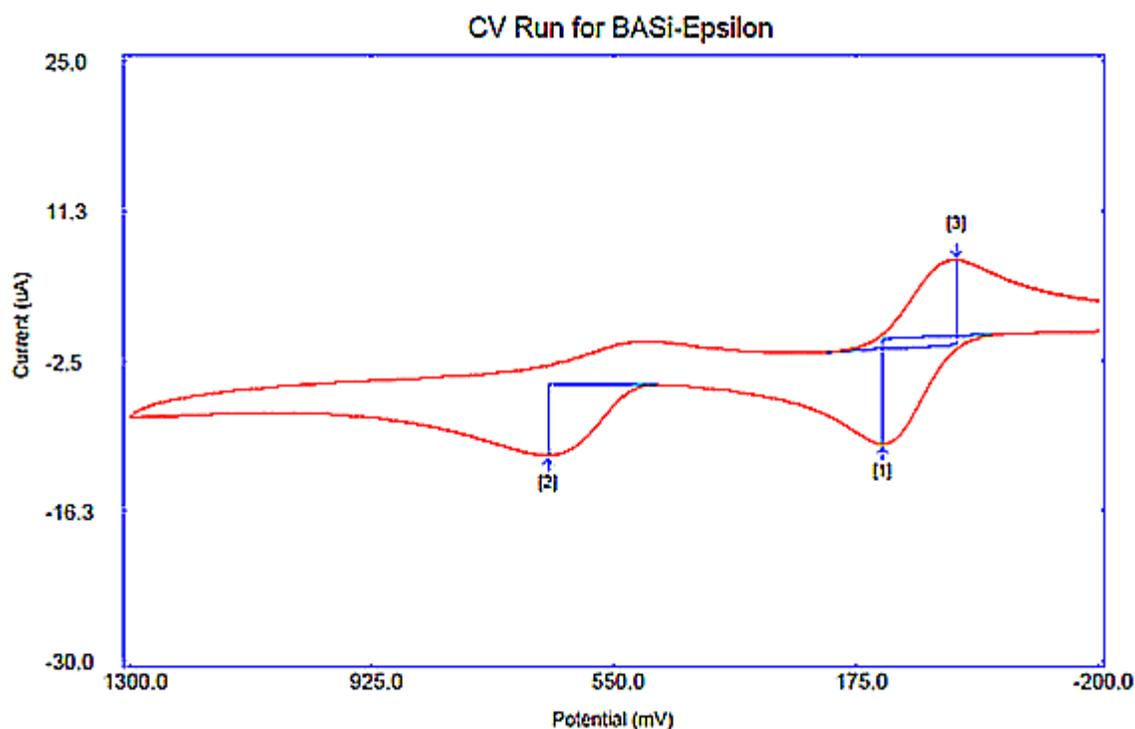
**Figure 11. Cyclic voltammogram for di-(4-*tert*-butylphenyl)-2-pyridylmethanamine with ferrocene internal standard.**
