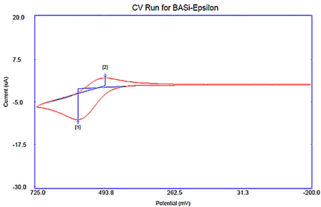
Figure 10. Cyclic voltammogram for di-(4-*tert*-butylphenyl)-2-pyridylmethylamine.
