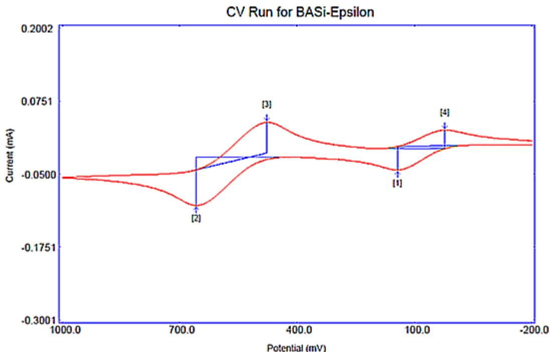
**Figure 6. Cyclic voltammogram for 2-chloro-10-(pyrid-2-yl)-10*H*-phenothiazine with ferrocene internal standard**
