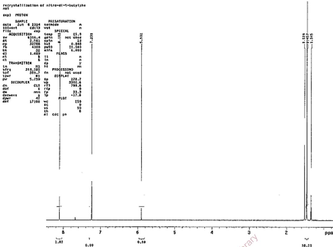
Figure 12. <sup>1</sup>H NMR spectrum of 4-nitro-2,6-di-*tert*-butylphenol.
