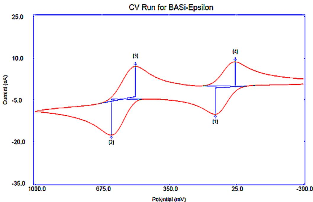
**Figure 9. Cyclic voltammogram for 10-(2-pyridinylmethyl)-2-trifluoromethyl-10H-phenothiazine with ferrocene internal standard.**
