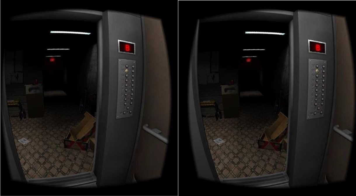
Figure 1. Sample of the offset between the digitally constructed images, each being projected into one of the retinas simultaneously allowing for 3D simulation.
